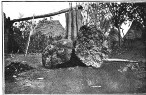
FIG. 9.—Two Pigs of Metal as they have come from the Cupola.
